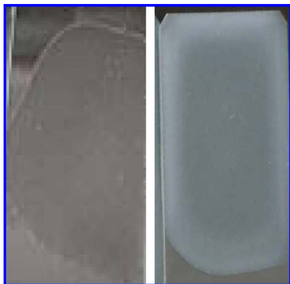
Figure 4. The photograph of P(VTMS/12FMA)-g-starch film (left) and VTMS-starch@P(MMA/BA/3FMA) film (right). [Color figure can be viewed in the online issue, which is available at wileyonlinelibrary.com.]
